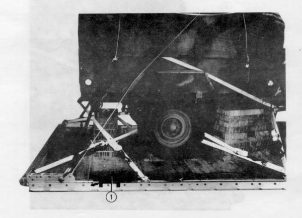
1 Install the components of the extraction force transfer coupling (EFTC) according to FM 10-500-2/TO 13C7-1-5. Use the forward mounting holes for the EFTC bracket.
