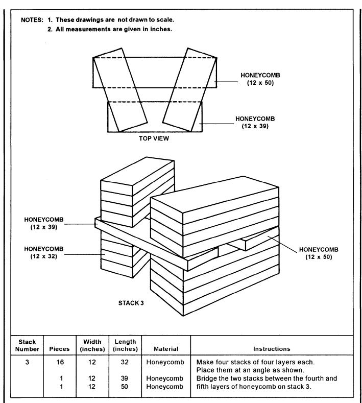
Figure 3-3. Honeycomb stack 3 prepared
