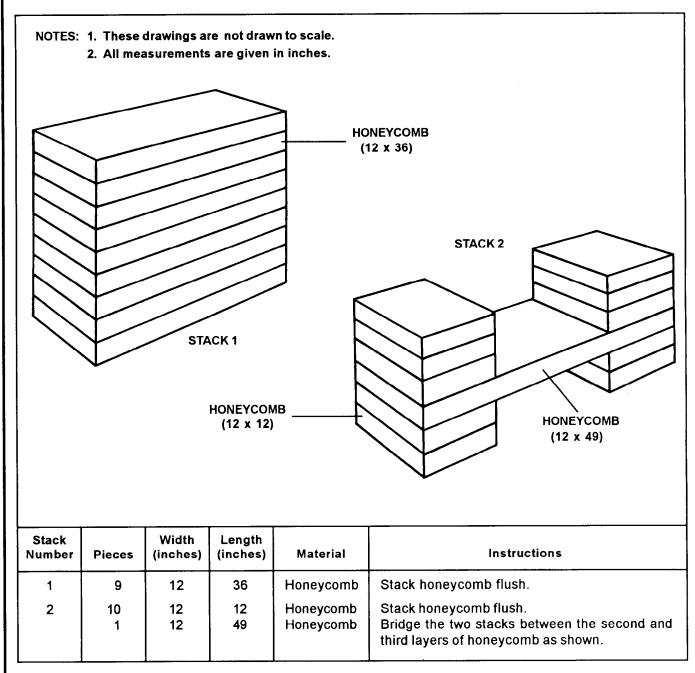
Figure 3-2. Honeycomb stacks 1 and 2 prepared
